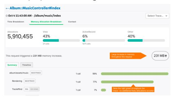
Method calls displayed in the trace details are organized from most to least allocations. The horizontal bar on the right visually represents the number of allocations associated with the method call(s) on the left. Some of the bars may have two shades of green: the lighter green represents the control case (what we view as a normal request) and the darker green represents the memory-hungry case.
