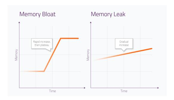
While memory bloat can quickly cripple a site, it's actually easier to track down the root cause than a memory leak.
